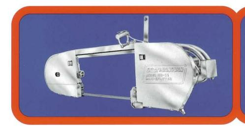
This high-performance bandsaw handles 150 cattle or 250+ hogs per hour and is equally well-suited for cattle, bulls, cows and hogs. The "150-SS" offers the sawyer an easy-handling perfectly balanced machine providing for accurate and straight splits. Equipped with a full 5-Horsepower [3.725 kw] waterproof heavy-duty motor, it is the most powerful bandsaw splitter available!
