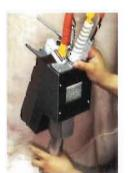
Using a simple, lightweight measuring head momentarily placed between the last and tenth rib, ACRA-Grade instantly generates an ultrasound image, while proprietary software automatically calculates total and percentage lean measurements. The operator can immediately confirm proper head placement and reliable data gathering. Data can be transmitted to a downstream scale for addition to the carcass weight report.
